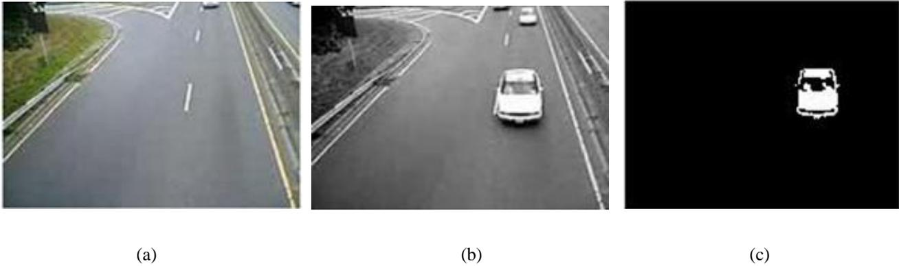
Fig. 2: a) Background Image b) After Gamma Correction c) After Subtraction
