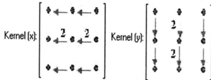
Fig. 3:  $S_x$  derivative in direction  $x$ ,  $S_y$  derivative in direction  $y$
