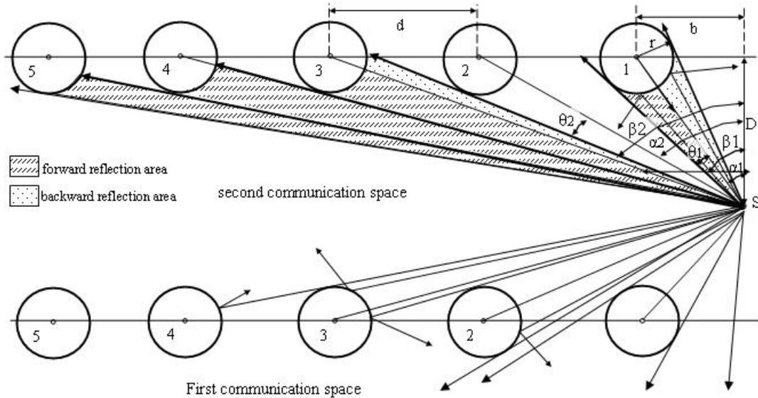
Fig. 3: Rays of single node between two communication spaces
