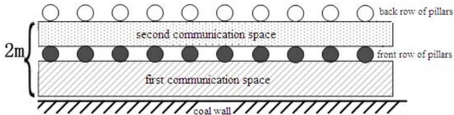
Fig. 2: Horizontal section of the coalface communication space
