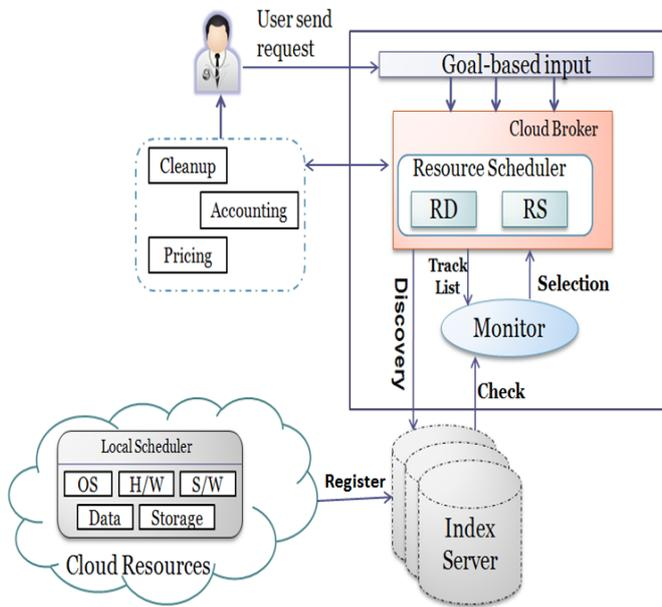
Fig. 1: Goal-based cloud broker architecture.
