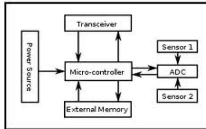
Fig. 1: Structure of sensor node
