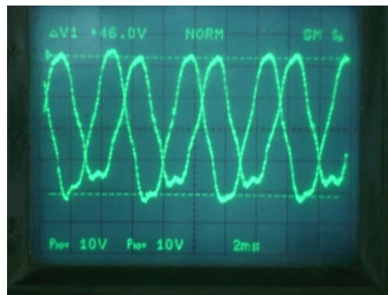
Fig. 4 AC voltage wave (phase difference  $120^\circ$ )
