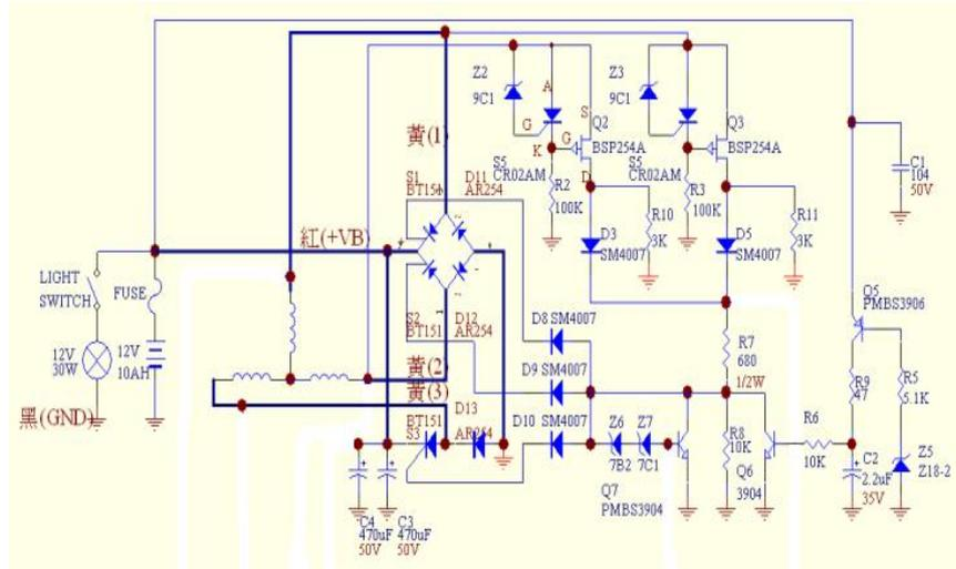
Fig. 2 Circuit of charging device
