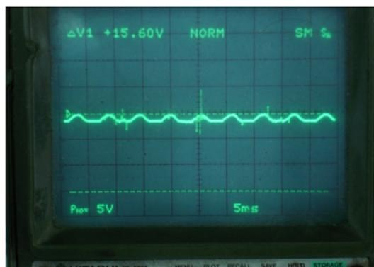
Fig. 5 Charging current 1.5 A, DC voltage of battery 13.9 V
