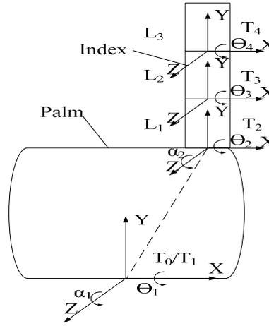
Fig.3. Simplified model of human hand motion
