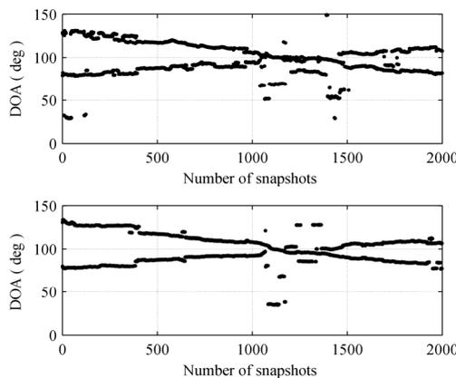
Figure 3. Comparison of DOA tracking results between before and after rejecting outliers, SNR=5dB
