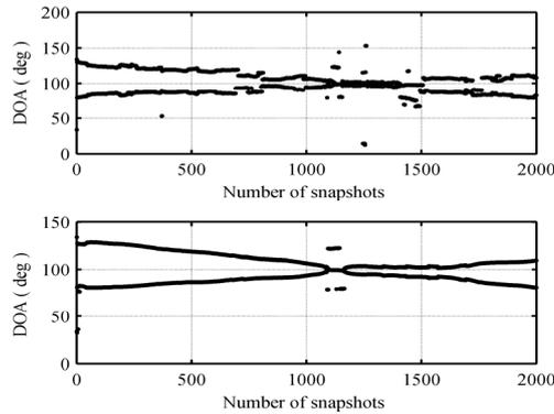
Figure 1. Comparison of DOA tracking results between before and after rejecting outliers, SNR=15dB
