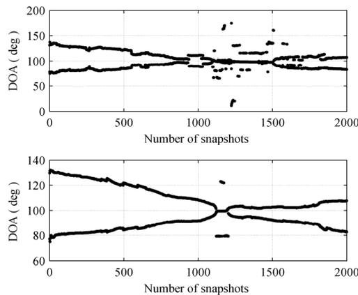
Figure 2. Comparison of DOA tracking results between before and after rejecting outliers, SNR=10dB
