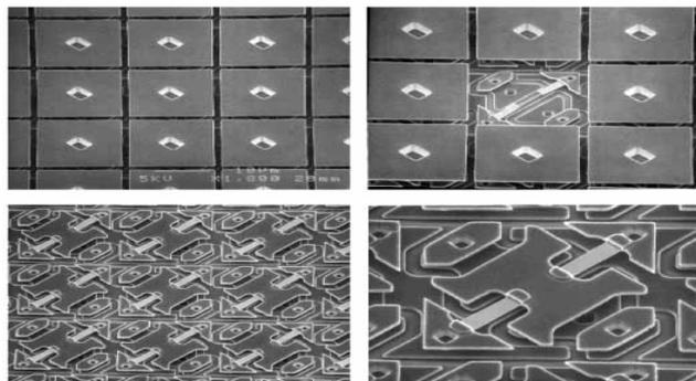
Figure 3. DMD mirror pictures by a Scanning Electron Microscope.
