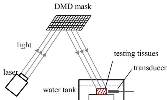
Figure 5. Schematic of CS photoacoustic imaging based on DMD
