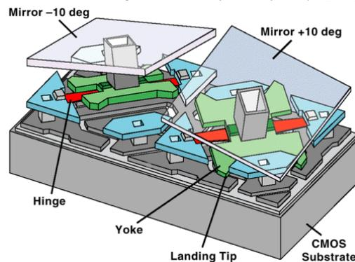
Figure 2. Schematic of the DMD mirror structure.
