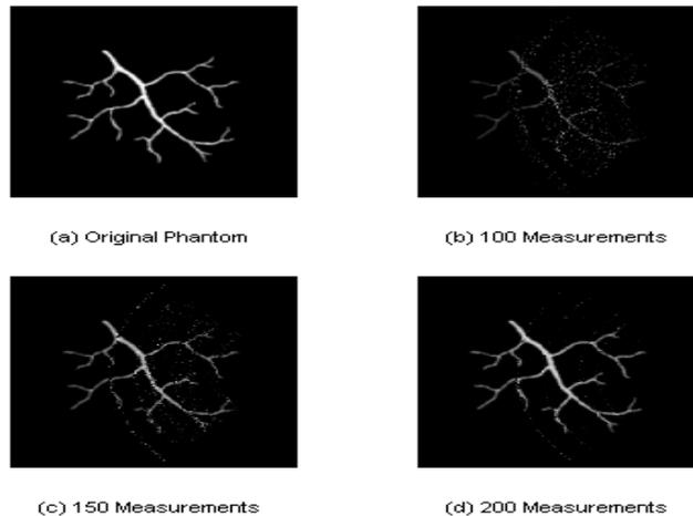
Figure 7. Reconstructed results for a photoacoustic phantom
