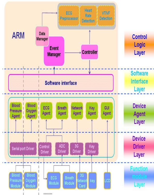
Fig. 1:Latticed model of telemonitoring system
