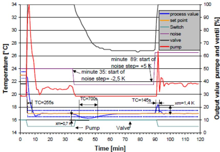
Fig. 5: Step response of the control Loop with two Actuators
