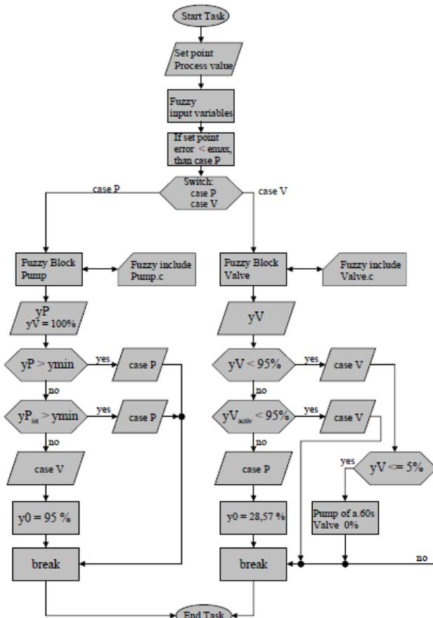
Fig. 3: Control Task for the Valve and the Pump
