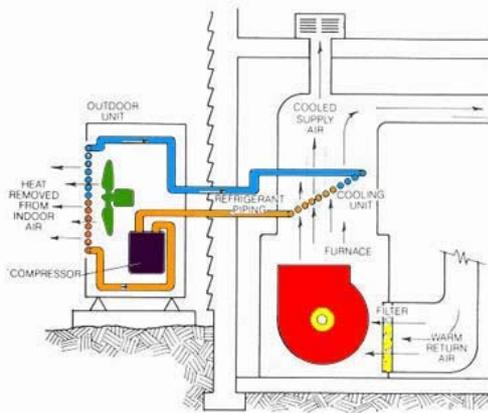
Fig 1. Work flow of a air-conditioning system
