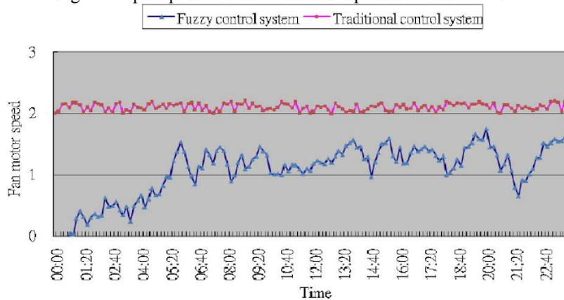
Fig. 6. The Fuzzy system performance with two actuators versus the traditional air-conditioning system
