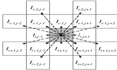
Fig. 1. A local configuration at the pixel position  $I_{i,j}$  for computing the variation  $V_c(I_{i,j})$ . The pixel  $I_{i,j}$  is marked as Gray Square.
