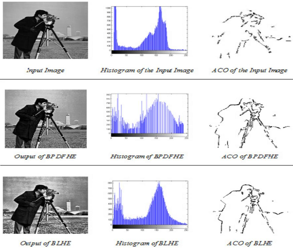
Fig. 4 Comparison of the input image, output of BPDFHE and output of BLHE, their histograms and also the edges detected using the ACO.
