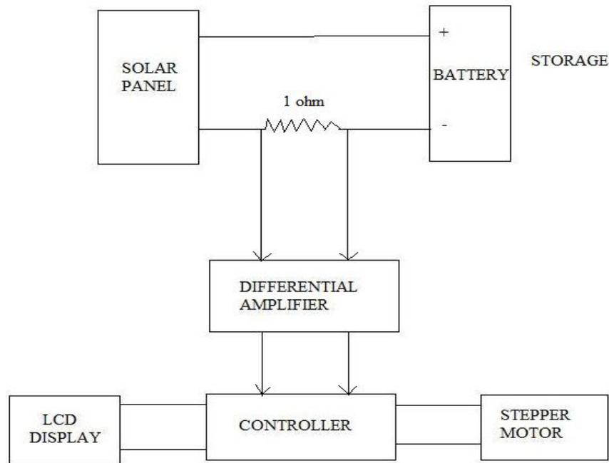
LCD (Liquid Crystal Display) is used in our proposed scheme to display the values of in-circuit current. For simulation purpose, we can use LCD in a 4-bit Mode. For that, we require only four data lines to be connected to the four port pins of PIC and three control signals to control the data flow and display.
