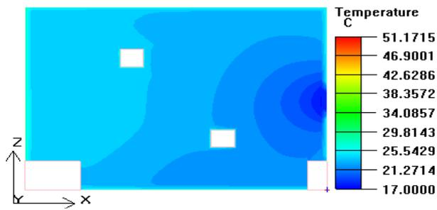
Fig.12  $T=17^{\circ}\text{C}, V=0.2\text{m/s}$ , the temperature field of the vertical section through  $(0, 0.1, 0)$
