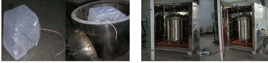
Fig.2. (a) Multilayer parcel in the low-pressure pot; (b) Airproof disposal and high-low temperature test chamber
