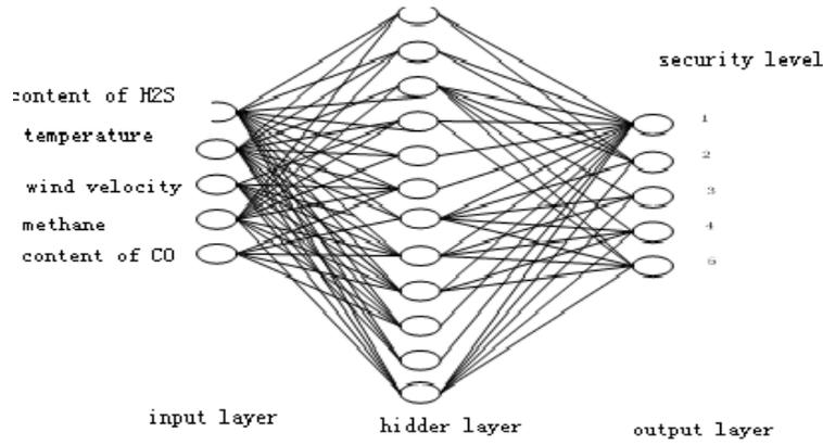
Fig 1: Multi-sensor information fusion of the neural network algorithm network model structure
