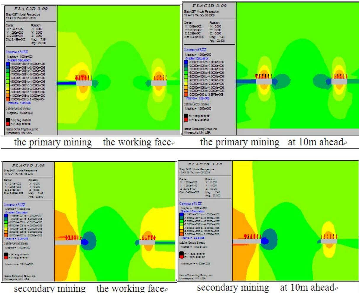
Figure 6 Vertical stress distribution at different position in the pillar under the influence by the mining when the pillar width is 20m
