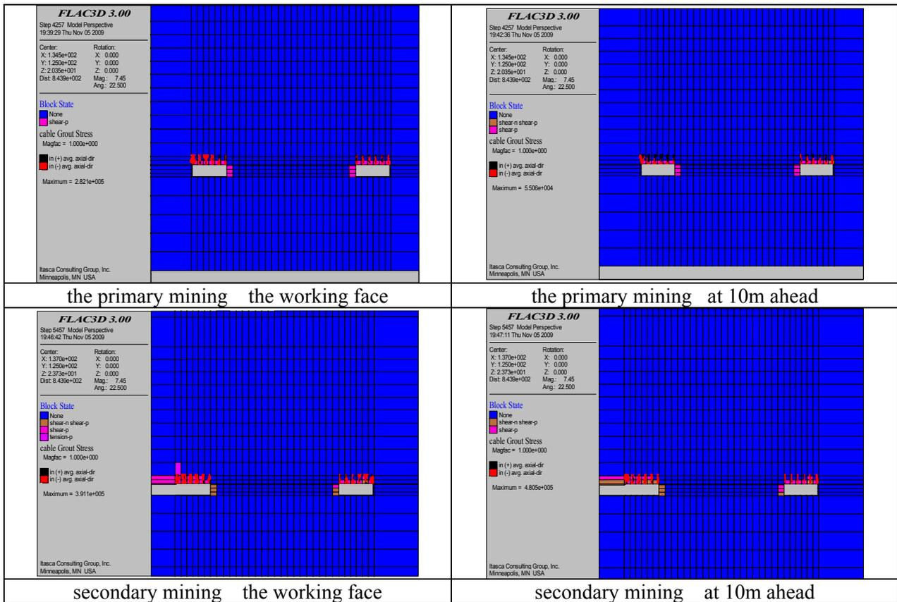
Figure 4 Different locations in roadway plastic failure figure when the width of the pillar is 20m under the influence of the mining
