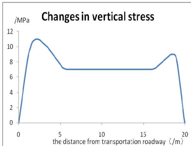
Figure 5 The vertical stress distribution of 20m pillar coal wall
