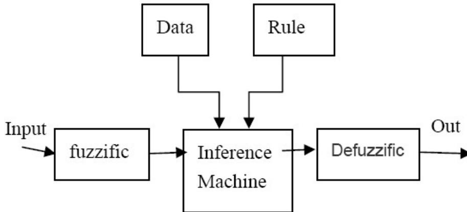
Diagram 3.1 the Structure Diagram of Fuzzy Evaluation System
