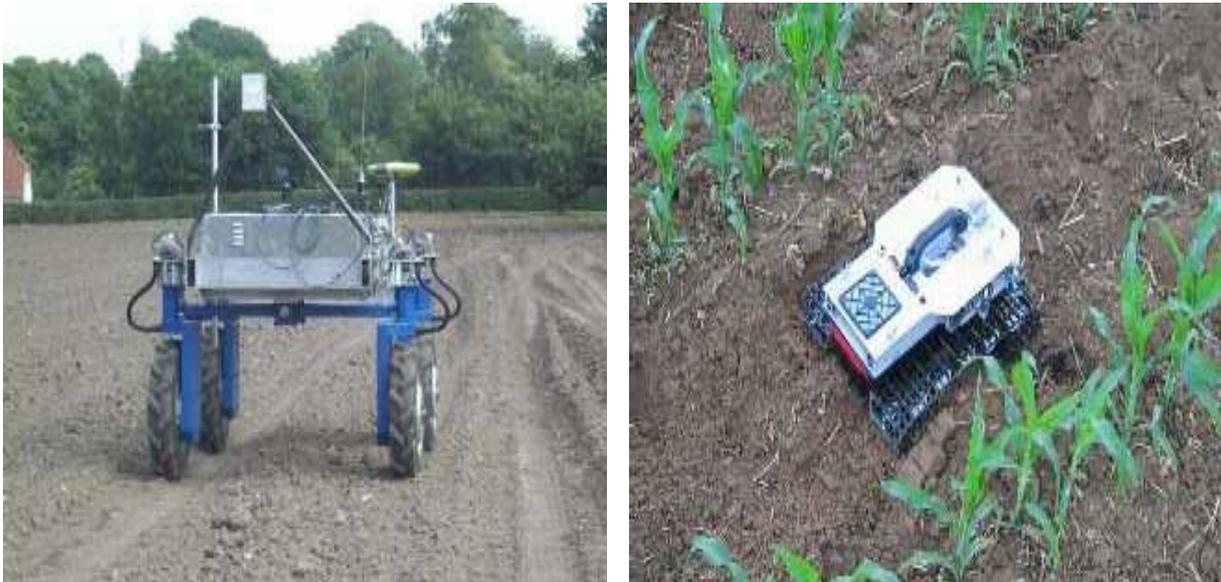
Fig 1. (Left) Portal crop scouting platform (Madsen and Jakobsen 2001), (Right) Sub canopy robot ISAAC2 built by a student team from Hohenheim University ([www.fieldrobot.nl](http://www.fieldrobot.nl))
