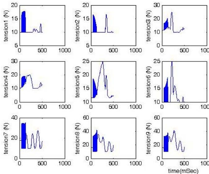
Fig. 5: Required cable tensions for circle tracking simulation at the presence of time-varying disturbances: Sliding Mode Control with PIID Sliding Surface
