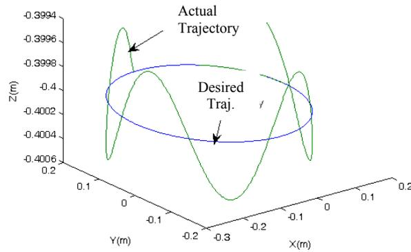
Fig. 3: Circle tracking simulation at the presence of time varying disturbance: PID-Computed Torque Control
