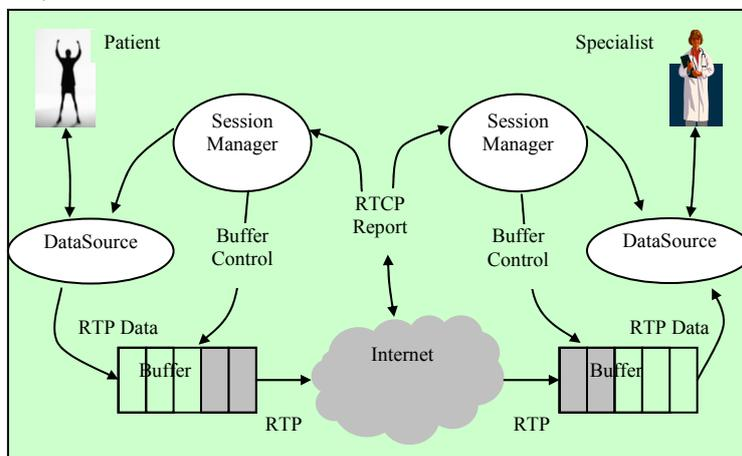
Figure 3. A streaming QoS control model
