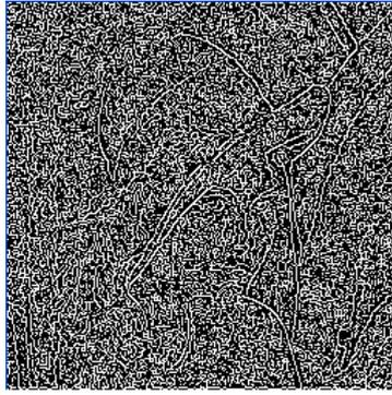
Figure 5. Processing Lena image with Canny operator
