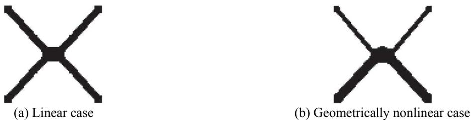
Fig. 7: Optimal topology using the BESO method
