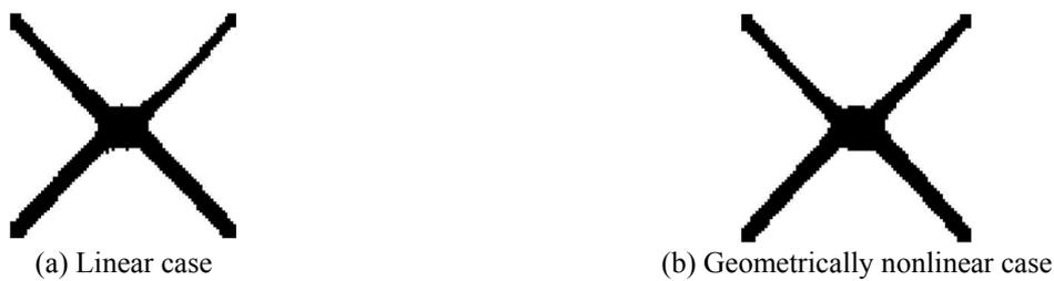
Fig. 6: Optimal topology using the modified ACO
