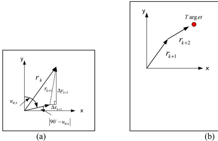
Fig. 2 (a) State transition from k to k+1; (b) 2-step control for WMR traveling to target at time k+2.
