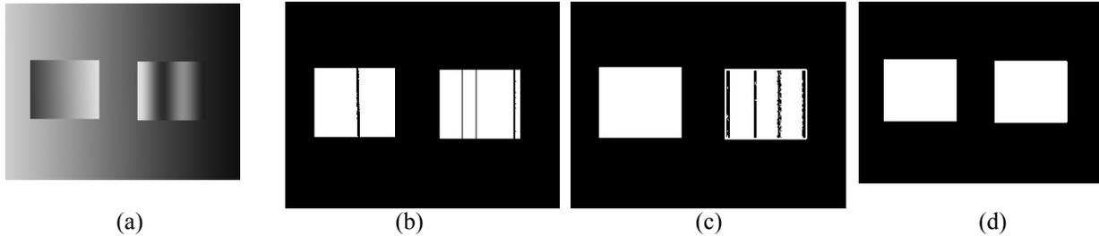
Fig. 2 (a) target image, (b) intensity threshold, (c) gradient threshold, and (d) combination of intensity and gradient threshold.
