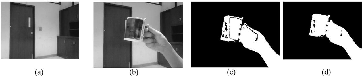
Fig. 3 (a) background image, (b) target image, (c) intensity threshold, and (d) combination of intensity and gradient threshold.
