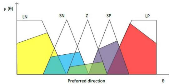
Fig.3. The final aggregated fuzzy sets for the preferred direction of the robot after the goal-enhancement is applied
