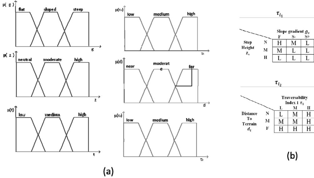
Fig.1. (a) Membership functions for inputs of slope gradient  $g_{si}$ , step height  $z_{si}$  and output Traversability Index 1  $\tau_{i1}$  and (b) Membership functions for inputs of Traversability Index 1  $\tau_{i1}$ , distance to terrain  $d_{ii}$  and output 2  $\tau_{i2}$
