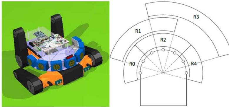
Fig.4. Image on the left shows the virtual agent, image on the right shows the regions corresponding to the cluster of ultrasonic sensors mounted on the robot for obstacle negotiation
