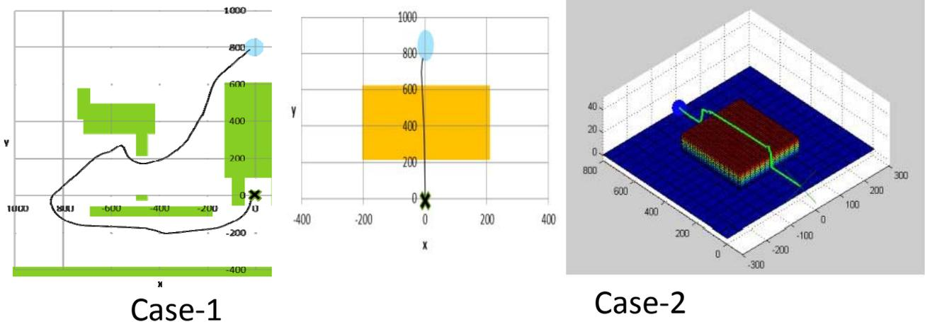
Fig.5. Case-1: Path taken by the virtual agent in the simulated environment; shaded regions represent obstacles. Case-2: Path taken by the virtual agent. Image on the left shows the robot on the 2D Cartesian plane while the image on the right shows the traversing in 3D space.
