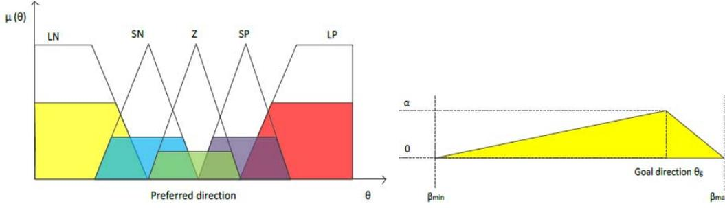
Fig. 2. (a) Aggregated fuzzy sets for the preferred direction of the robot (b) Illustration showing the magnitude of the additional multiplier with respect to the goal. and  $\beta_i$  represent the boundary for which the influence of the goal should reach in the universe of discourse of  $\theta$ .
