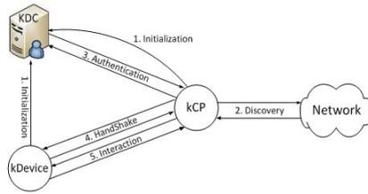
Fig. 1: Working mechanism of KUPnP
