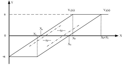
Fig.2 Transfer function curve of folder and interpolating signals
