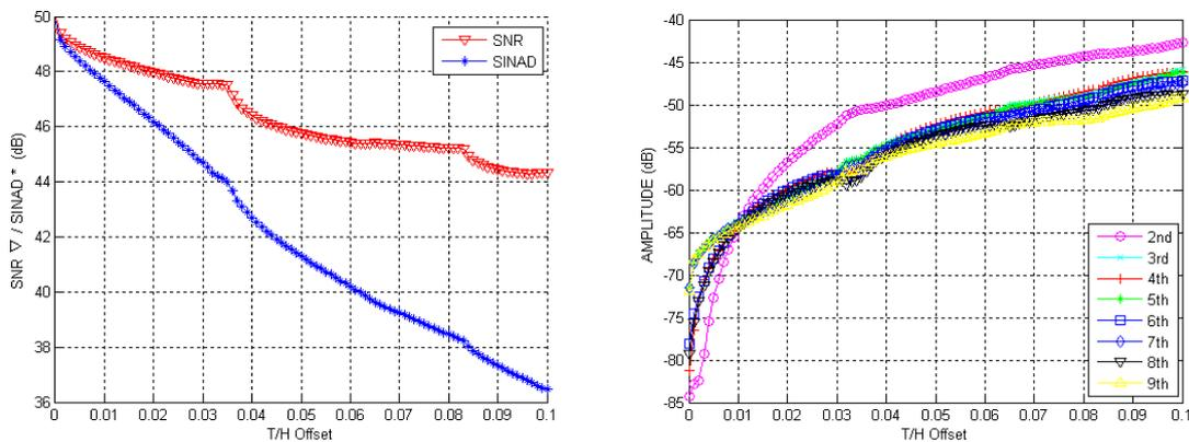
Fig. 6 SNR, SINAD and harmonic distortions versus T/H output bias
