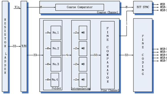
Fig. 3 8bit FIADC architecture
