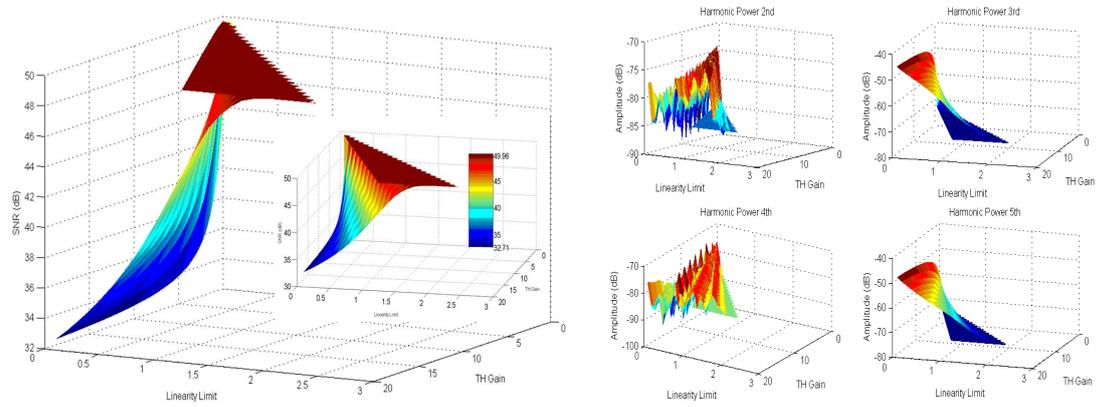
Fig. 7 SNR and harmonic distortions versus linear range and gain
