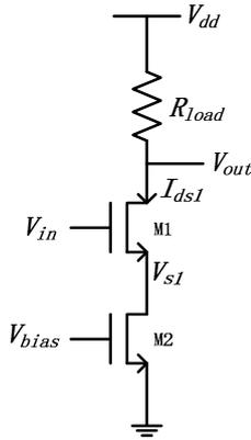
Fig.1 Common-source amplifier
