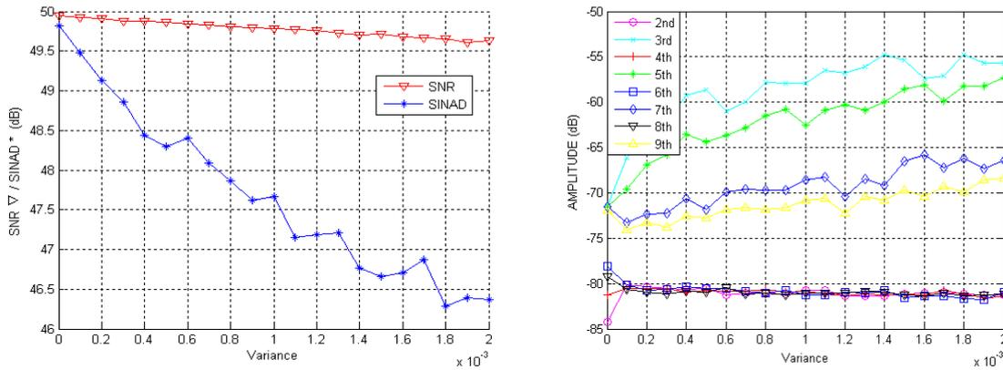
Fig. 5 SNR, SINAD and harmonic distortions versus resistor jitter
