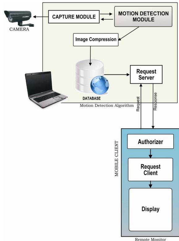
Fig. 1. Overall Architectural diagram.
