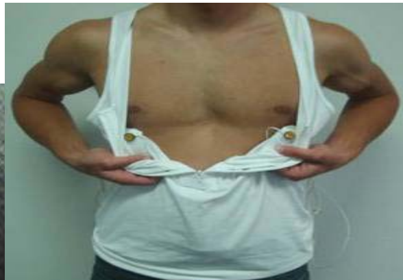
Fig.3 (b) Sensors attached on a T-shirts and Worn on a human body
