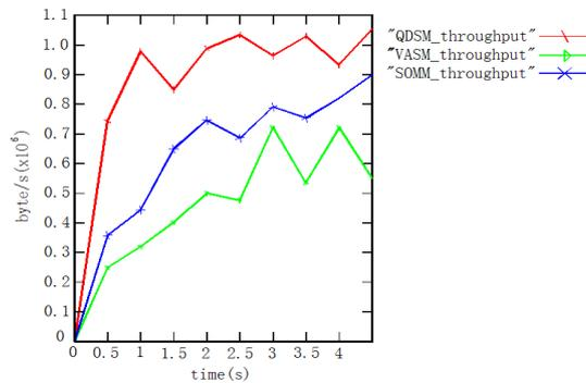
Figure 5. The throughput of QDSM, SOMM and VASM
