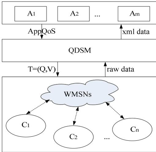
Figure 1. The WMSNs architecture based on QDSM
