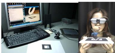
Figure 6. Web Camera Based and HMD Based of AR Project
