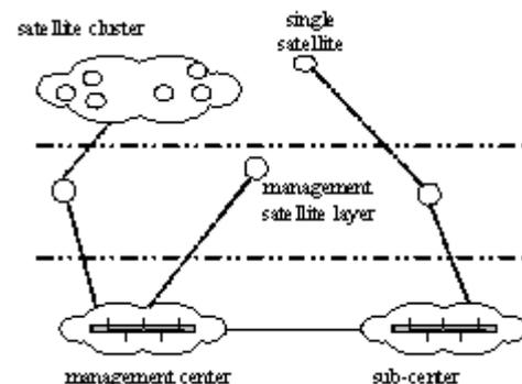
Figure 4 The Layered Architecture of Satellite Network Management
