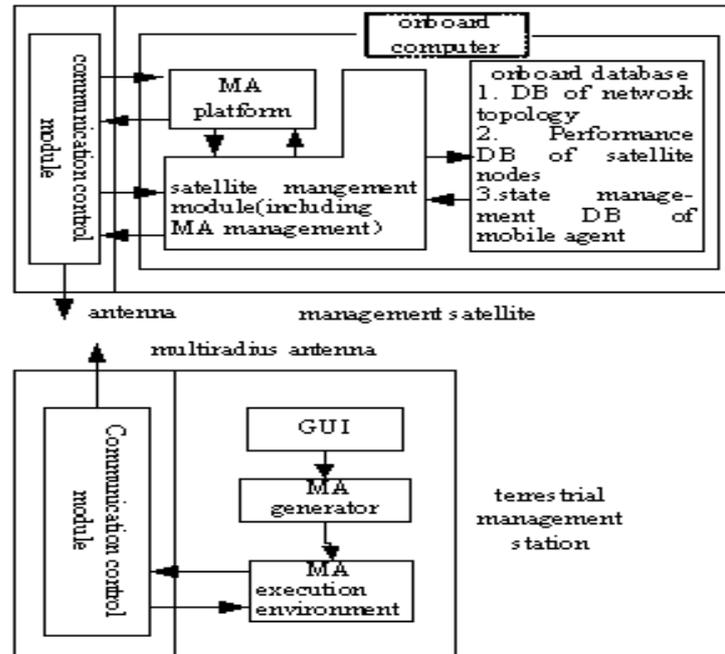
Figure 5 The System Architecture of Satellite Network Management
