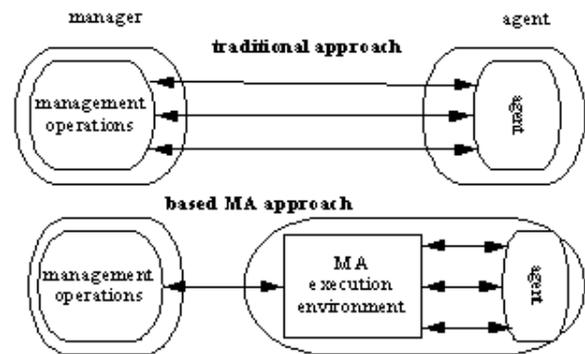
Figure 2 Mobile Agents Reduce Network Load
