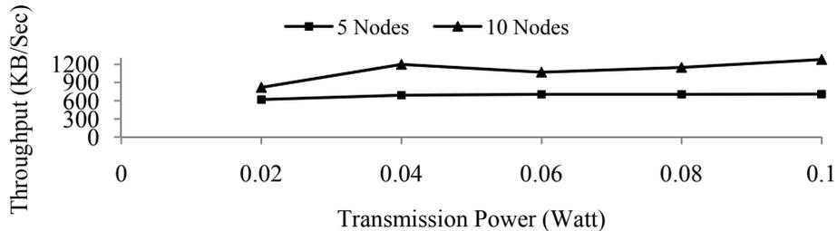
Fig. 7: Transmission power Vs Throughput
