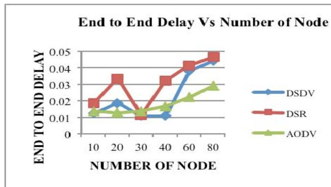
Fig. 2: End to End Delay Vs Number of Nodes for DSDV, DSR and AODV
