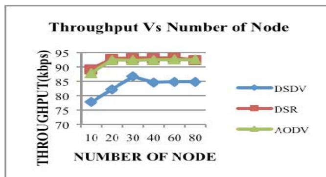
Fig. 4: Throughput Vs Number of Nodes for DSDV, DSR and AODV
