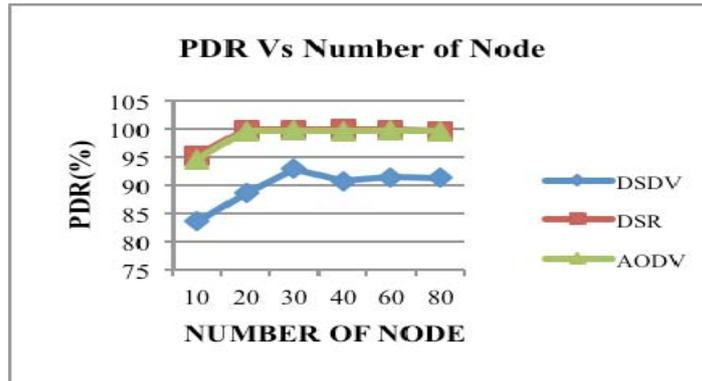
Fig. 1: Packet Delivery Ratio Vs Number of nodes for DSDV, DSR and AODV
