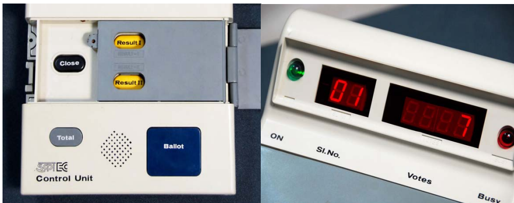
Fig. 2: Counting Votes—The EVM records votes in its internal memory. At a public counting session, workers remove a seal on the control unit and press the RESULT I button (left) to reveal the results. The machine sequentially outputs the number of votes received by each candidate using a bank of 7-segment LEDs (right). Here, candidate number 01 has received 7 votes.
