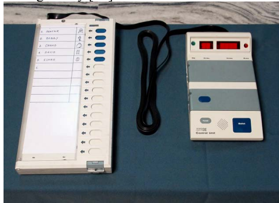
Fig. 1: Indian EVMs consist of a BALLOT UNIT used by voters (left) and a CONTROL UNIT operated by poll workers (right) joined by a 5-meter cable. Voters simply press the button corresponding to the candidate of their choice.
