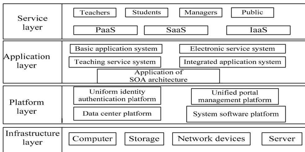
Fig. 2 The digital campus system structure of cloud computing based on SOA
