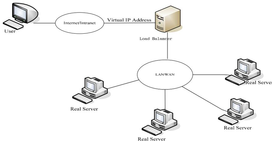
Fig. 1 The architecture of Virtual server
