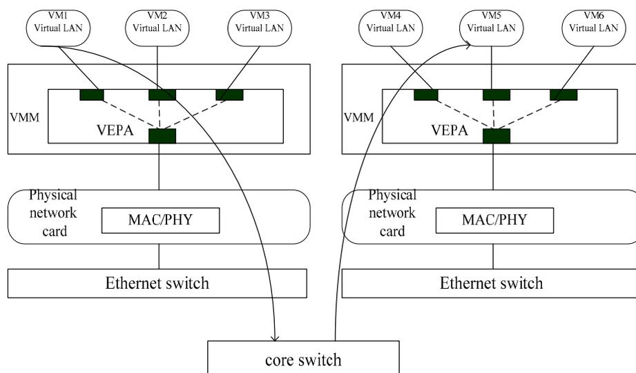
Fig. 4 the working principle of VEPA
