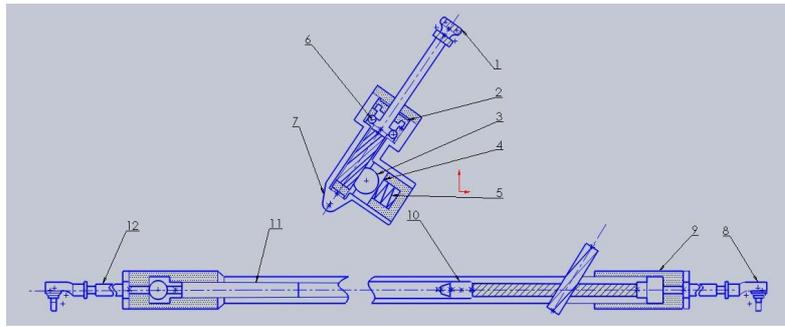
1.small gear 2. oil seal 3. rack 4. block 5. spring 6. bearing 7. steering shell
