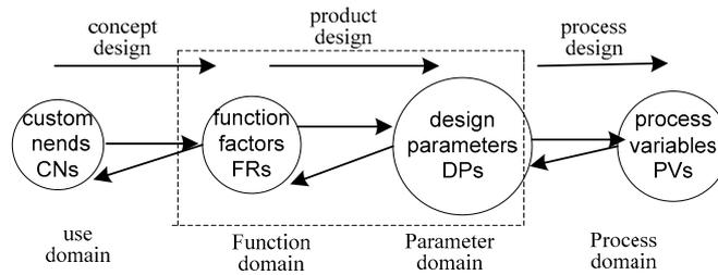
Fig.1 The Relation of Four Domains in Axiomatic Design
