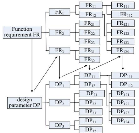
Fig.3 Decomposition of Function Requirement and Design Parameter for Steering
