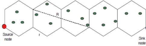
Fig. 1: Equal-cell GAF model.
