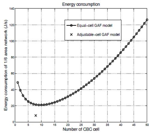
Fig. 4: Comparison of energy consumption.
