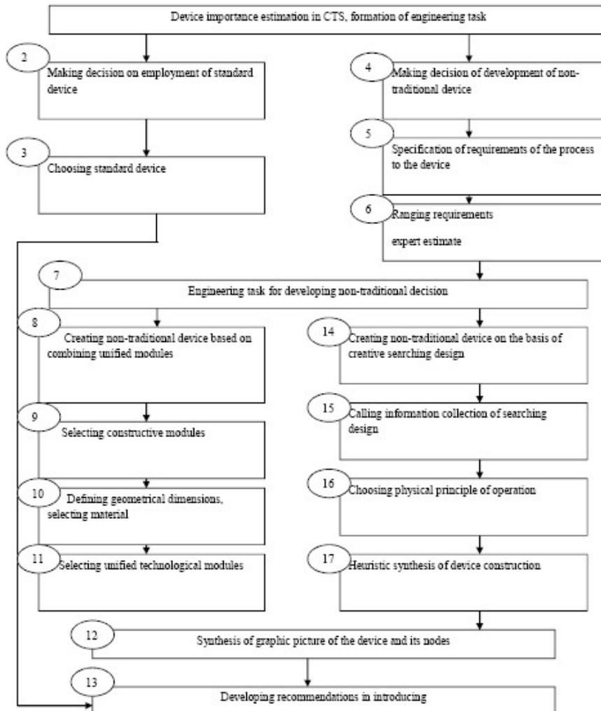
Fig 1. Logical block-scheme of the algorithm of choice and design of the device for CTS
