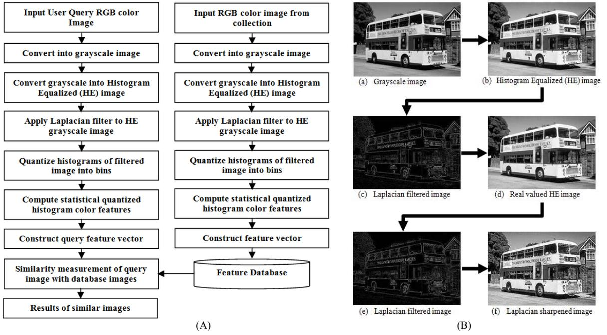
Fig. 1. (A) Block diagram of the proposed algorithm (B) Sharpening process using Laplacian filter
