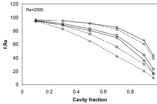
Fig. 5: The friction factor-Reynolds number product versus cavity fractions at different values of relative module width,  $W_m = 0.1$  (circle),  $W_m = 0.5$  (square) and  $W_m = 0.9$  (triangle). Solid and dashed lines are associated with the staggered and aligned configurations, respectively.
