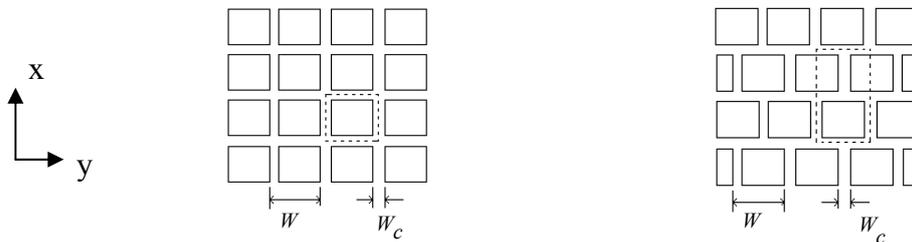
Fig. 2: Two different patterns of superhydrophobic surface viewed from the top.
