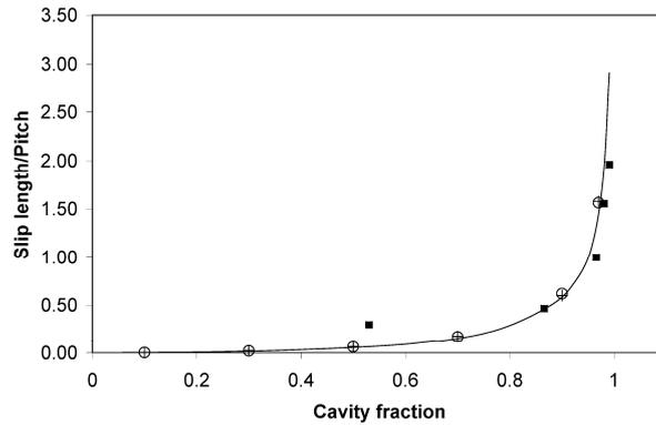
Fig. 4: Normalized slip length for present study and those reported in the literature. Present study (aligned (+) and staggered (O) microposts), theory of Ybert et al. [5] (solid lines) and experimental results [17] (solid square).
