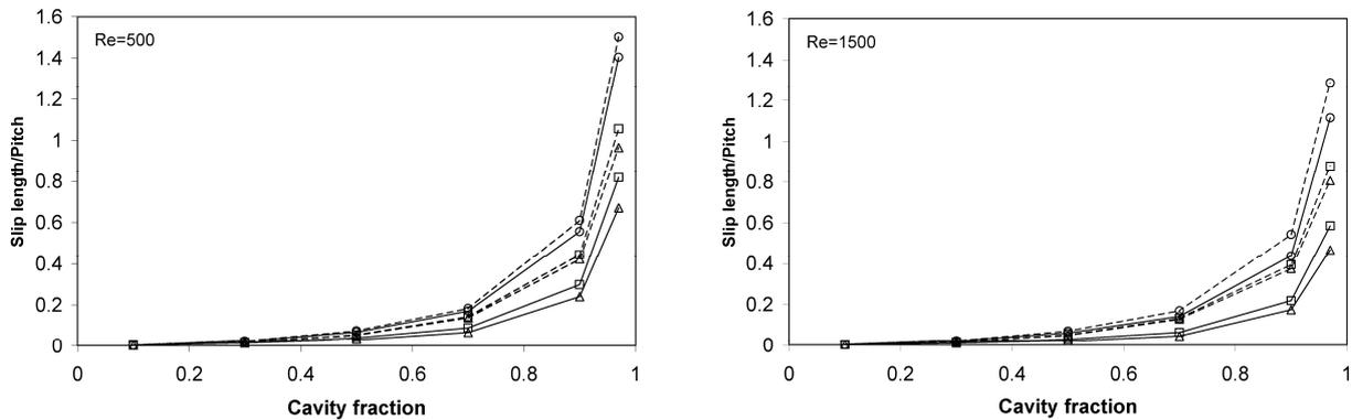
Fig. 6: The non-dimensional slip length versus cavity fractions at different values of relative module width,  $W_m = 0.1$  (circle),  $W_m = 0.5$  (square) and  $W_m = 0.9$  (triangle). Solid and dashed lines are associated with the staggered and aligned configurations, respectively.
