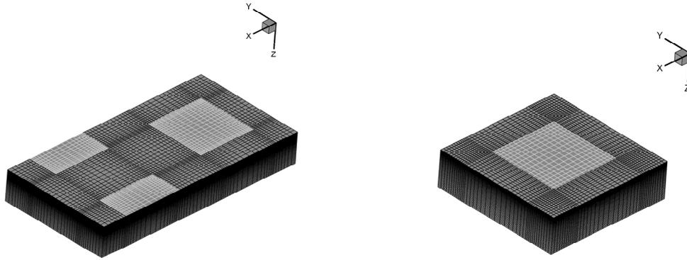
Fig. 3: Two typical grids used for numerical calculations for staggered (left) and aligned (right) configurations.
