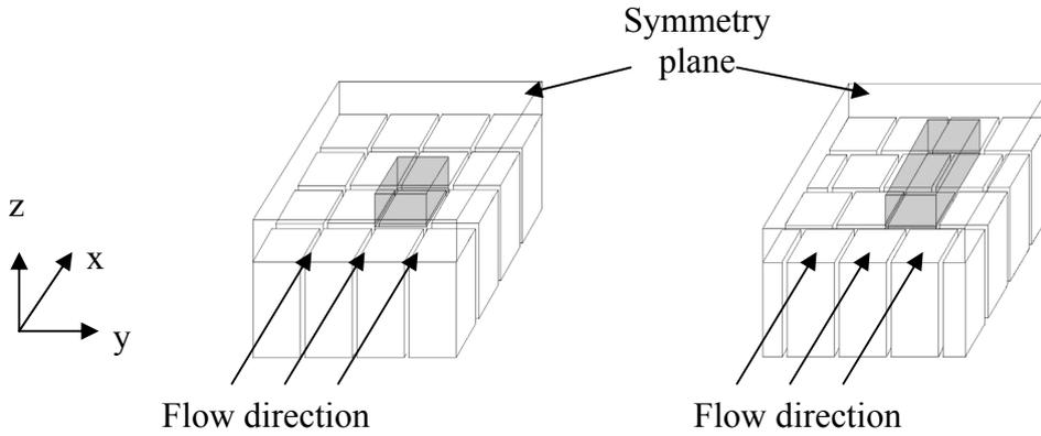
Fig. 1: The aligned (left) and staggered (right) microposts used as the microchannel walls.
