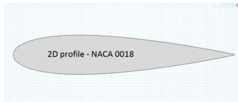
Figure 1: Two dimensional NACA 0018 profile made by using X and Y coordinates.
