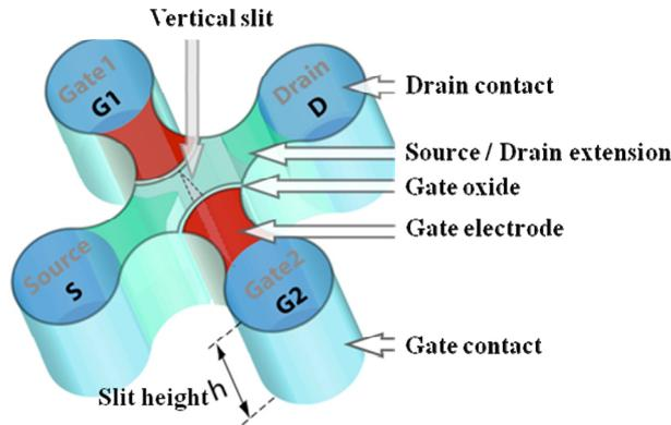
Fig. 1: Schematic drawing of junction-less VeSFET, with circularly-designed source/drain and gates that can be printed without complex OPC. The contact plugs to source /drain and gate can be through the top silicon to make the device vertically homogeneous and thus allowing interconnects from both sides.
