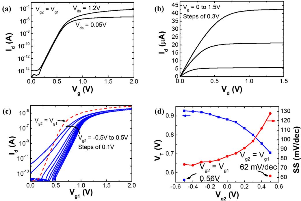
Fig. 3: (a)  $I_d$ - $V_g$  and (b)  $I_d$ - $V_d$  characteristics when both gates are swept together, showing no short-channel effects, (c)  $I_d$ - $V_g$  characteristics when Gate 1 is swept while Gate 2 is biased ( $V_{ds}=1.2\text{V}$ ). The red dotted line represents the  $I_d$ - $V_g$  curve when both gates are swept together. (d) Threshold voltage ( $V_T$ ) and SS variation when Gate 2 is biased.  $V_T$  extraction is through linear extrapolation method.
