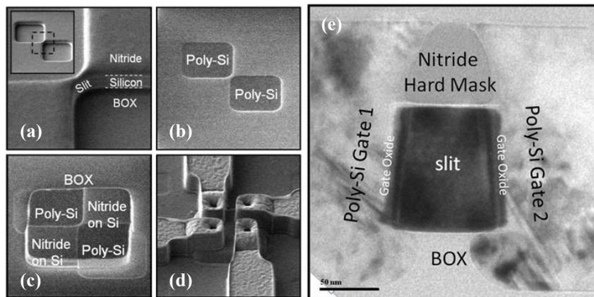
Fig. 2: Tilted SEM images after (a) nitride hard mask etch and silicon slit etch, (b) poly-Si gate CMP, (c) source/drain isolation etch and (d) metallization with four terminals. (e) Cross-sectional TEM image across a VeSFET device slit, showing the two independent gates on either side of the silicon slit.
