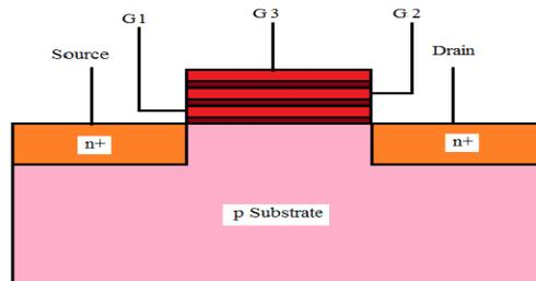
Fig. 1: Variable gate oxide thickness MOSFET
