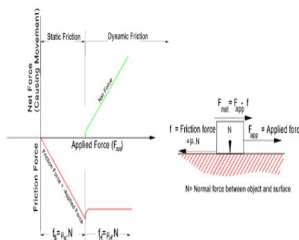
Fig. 1: Principle of COF Testing
