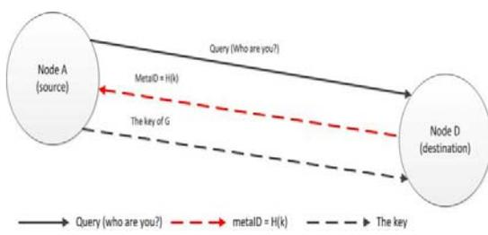
Fig. 3: Hash lock scheme on AODV protocol
