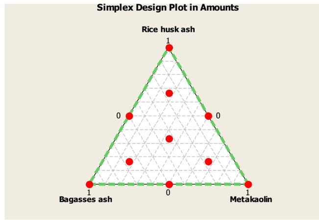
Fig.1 Design of experiment as Simplex Centroid of pozzolan material proportion
