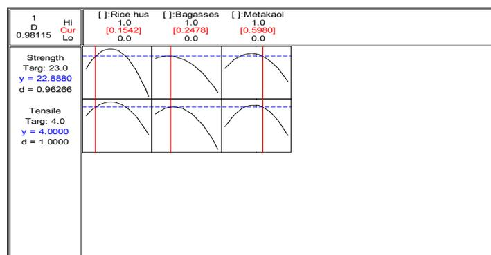
Fig.4 Response and desirability of compressive strength and tensile strength
