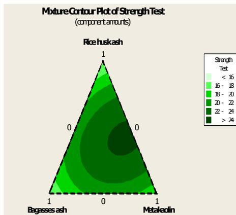
Fig.2 Response mixture of compressive strength testing
