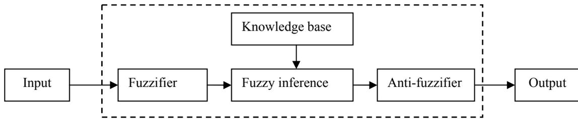
Fig. 1: The Structure of Fuzzy Inference System
