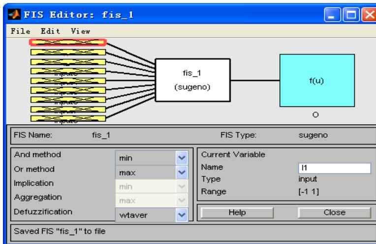
Fig. 3: The fuzzy inference system for fault diagnosis
