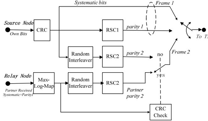
Fig. 1: Turbo encoding in a coded cooperation scheme
