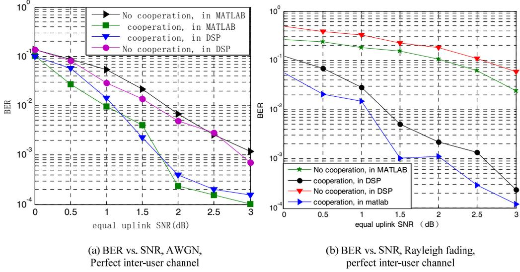
Fig.4: BER curves simulated in AWGN and Rayleigh fading channel
