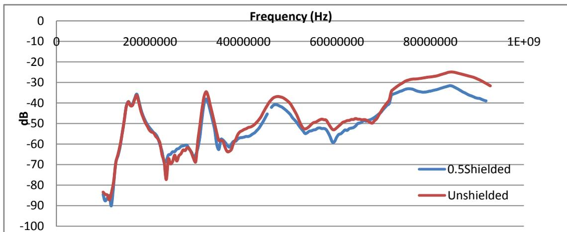
Fig. 1: Measurement of shielding effectiveness of 0.5 inch Mu-Metal.
