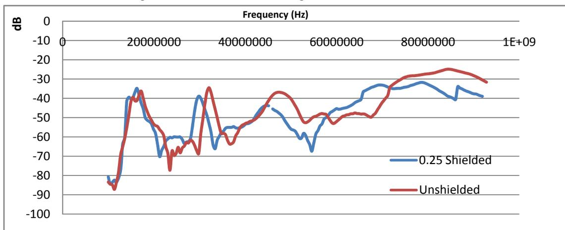
Fig. 2: Measurement of shielding effectiveness of 0.25 inch Mu-Metal.
